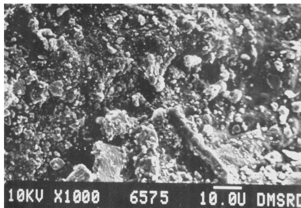
Figure 4 SEM photograph of carbon black + phenolic resin filled vulcanizate of mix D.
